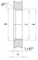
Installation direction: o-ring sits on chamfer.
